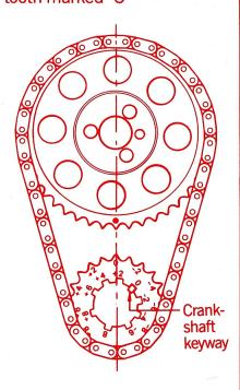
**Warning:** Do not use the keyway marks to time engine. Always align the crank gear tooth timing mark to cam gear timing mark.
